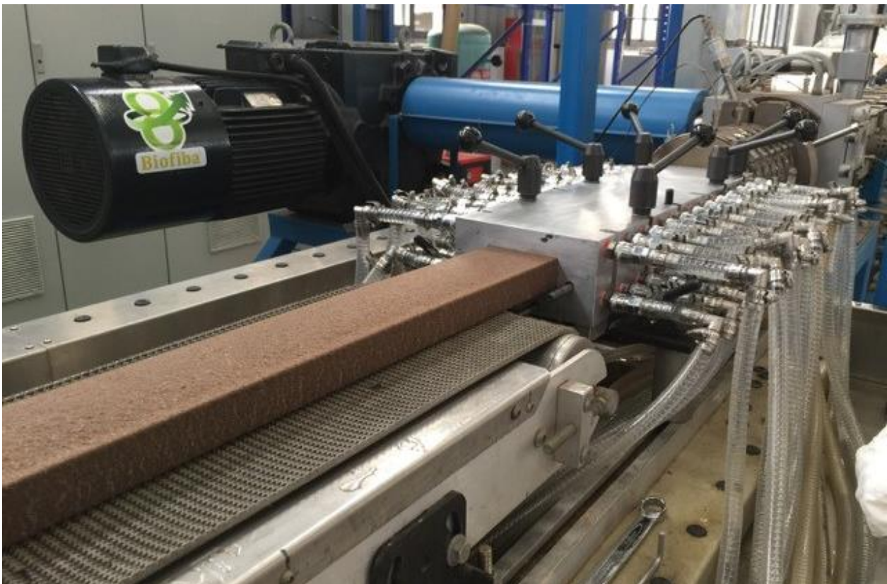
Biofiba® profile extrusion line at production facility in Zhoushan, China.
